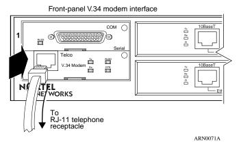
Figure 1-1. ARN V.34 Modem Adapter Module Connector (Slot 2)
